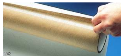
High tack side of 3M™ Removable/Repositionable Tape 9415 “permanently” adheres to cores for winding up paper or film. Low tack side releases the paper or film when unwinding.
