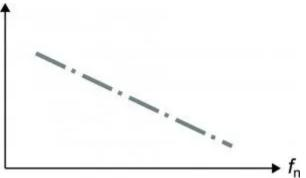
Feed,  $f_{n}$ , has less effect on tool life than  $v_c$ . (Tool life on Y-axis)
