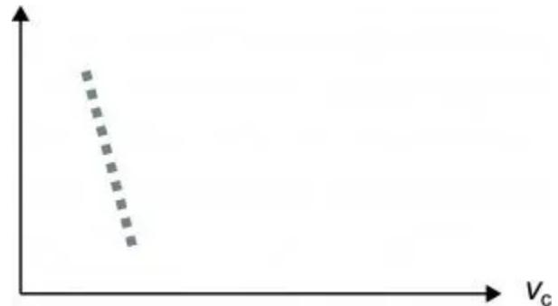
Cutting speed,  $v_c$ , has a significant effect on tool life. Adjust  $v_c$  for best economy  $v_c$ .
