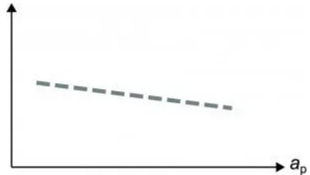
Depth of cut,  $a_p$ , has a small effect on tool life.
