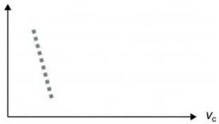
Cutting speed,  $v_c$ , has a significant effect on tool life. Adjust  $v_c$  for best economy  $v_c$ . (Tool life on Y-axis)
