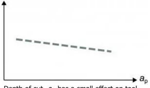
Depth of cut,  $a_p$ , has a small effect on tool life. (Tool life on Y-axis)
